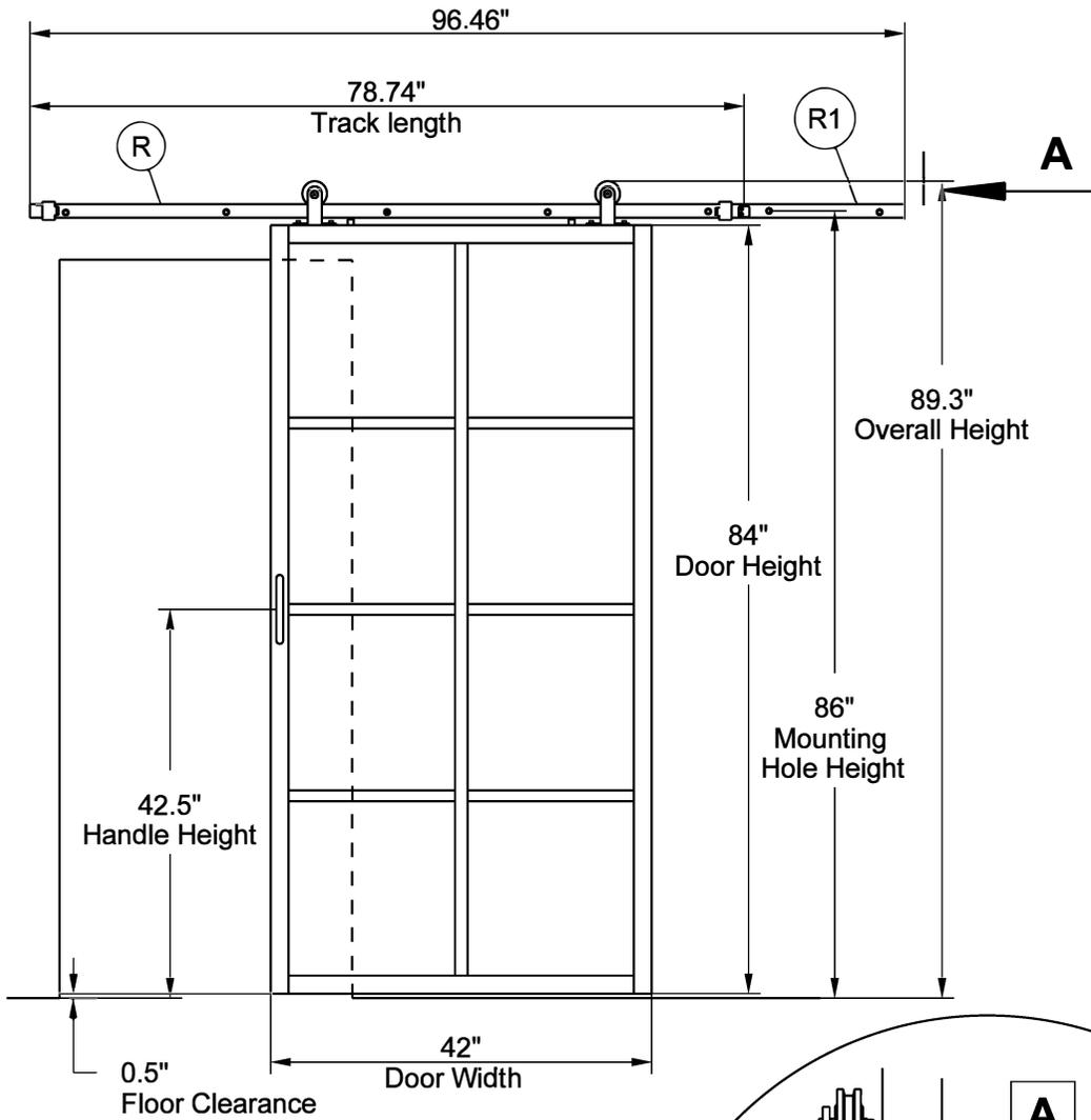
Door is Reversible Handing. Determine which way the door will open prior to hanging the door and installing the handle.
